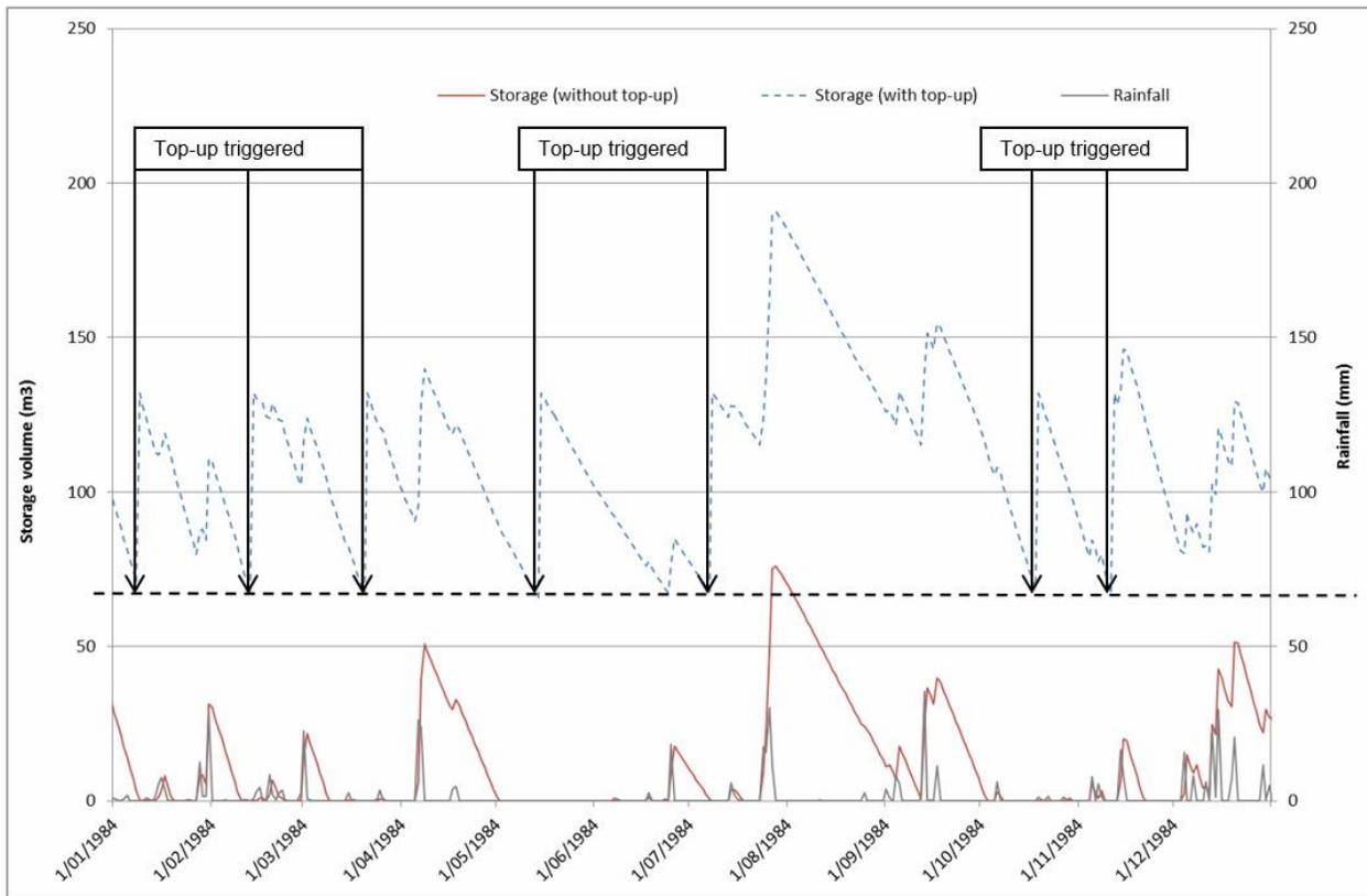
**Figure 5. Storage volume comparison for wicking bed, with and with-out top up for one of the driest modelled years (annual rainfall 547 mm), highlighting how top-up helps to sustain storage volumes during dry years.**
