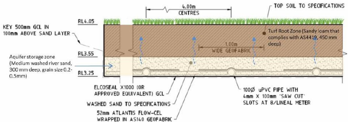
**Figure 1. Typical section through wicking bed.**
