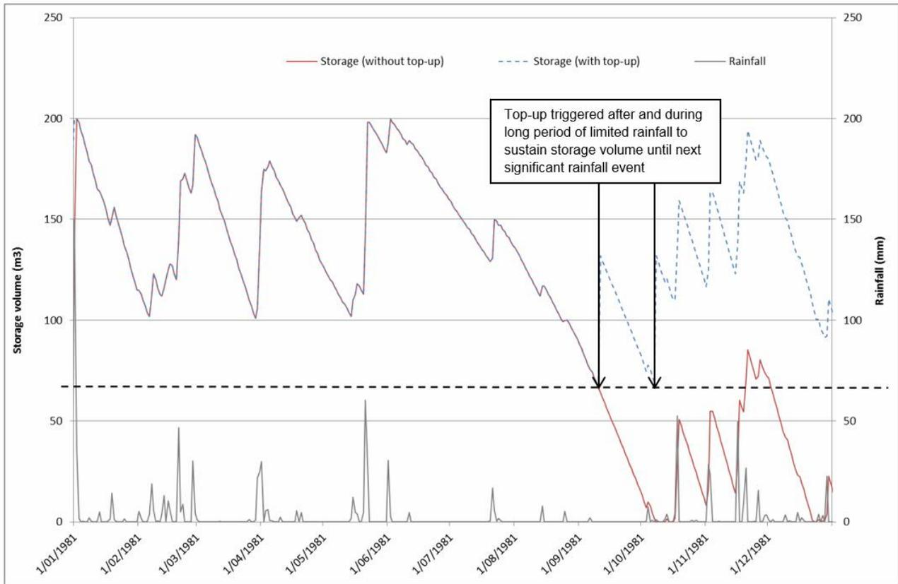
**Figure 4. Storage volume comparison for wicking bed, with and with-out top up for one of the modelled years with an average rainfall (966 mm), highlighting how top-up helps to sustain storage volumes during periods of low rainfall.**
