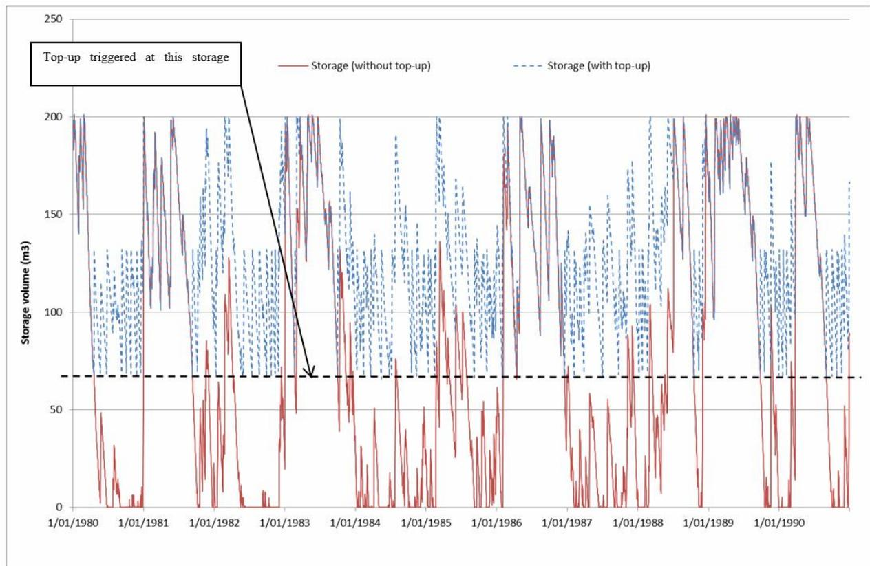
**Figure 3. Storage volume comparison for wicking bed, with and with-out top up.**
